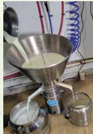
The Milky FJ 350 Separator can generate 92 gallons per hour.
