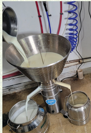
The Milky FJ 350 Separator can generate 92 gallons per hour.
