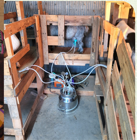
Special accessory lid to milk three goats or sheep at once. (See page 18)
